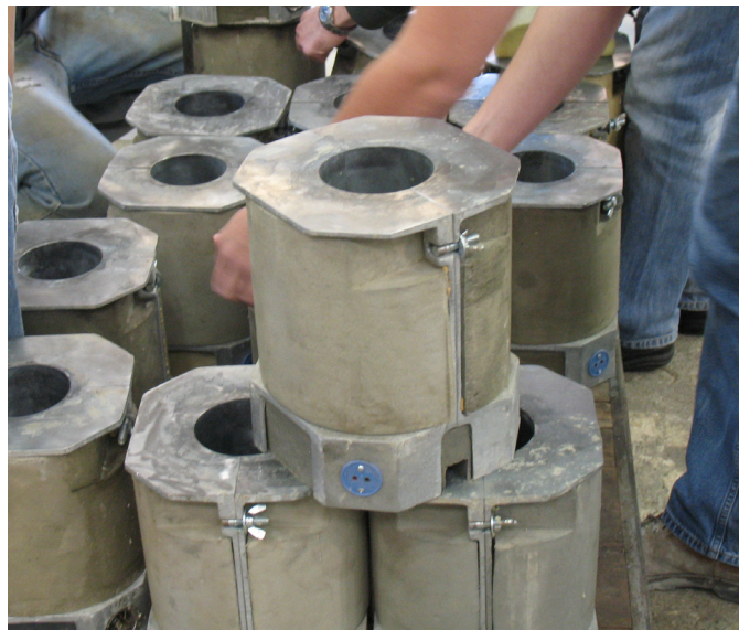
Figure 3- 15: Match Curing Cylinders
