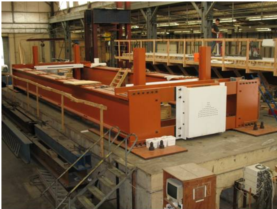
Figure 3- 11: FSEL High Capacity Prestressing Bed (O'Callaghan, 2007)
