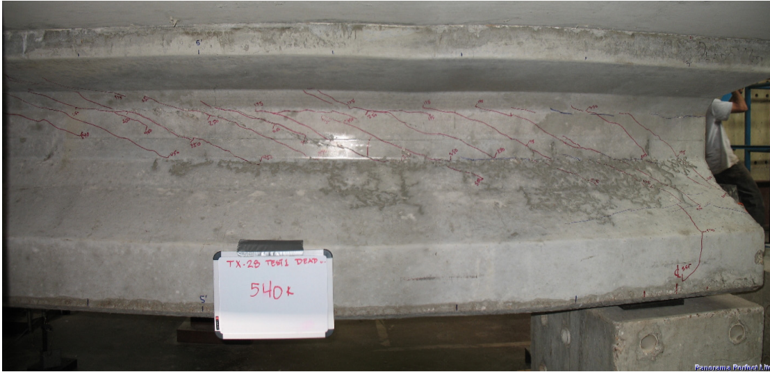
Figure 4- 28: Dead end of Tx28-I at failure for Test 3.
