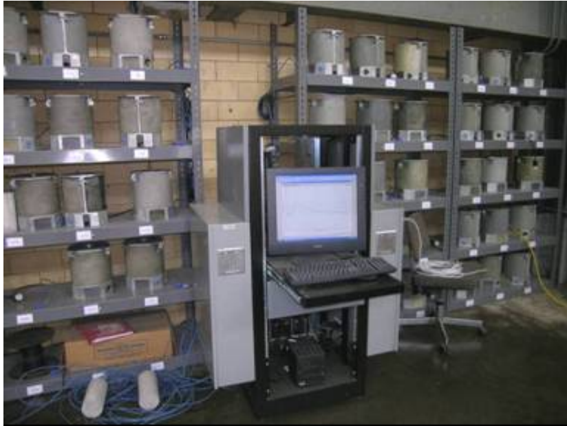
Figure 3- 14: Match Curing Controller and Cylinders (O'Callaghan, 2007)
