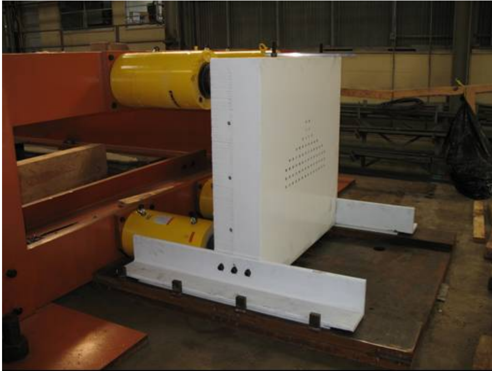
Figure 3- 12: Live End Bulkhead and set of 4 hydraulic rams. (O’Callaghan, 2007)
