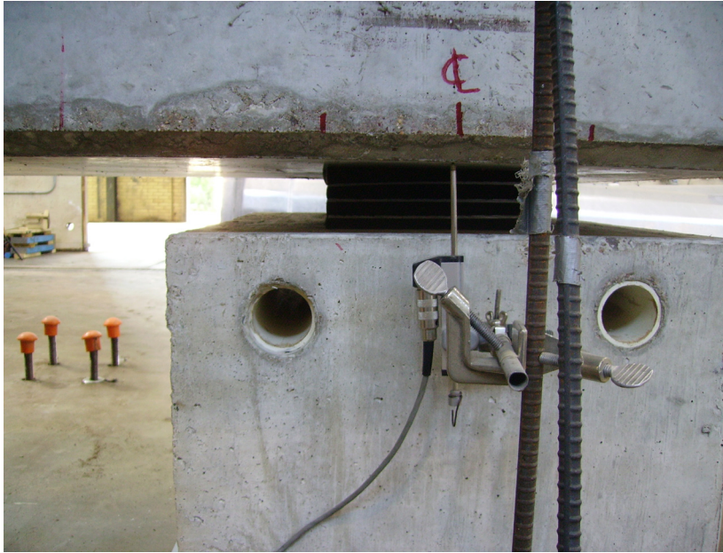
Figure 3- 9: 2" Linear Potentiometer at the support.
