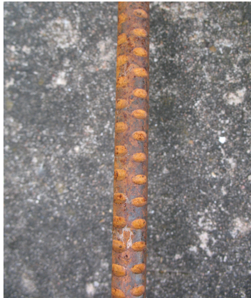
Figure 3- 3: Prefabricated welded-deformed rebar
